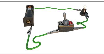
When electricity flows through all the components of a circuit, it is called a complete circuit.
